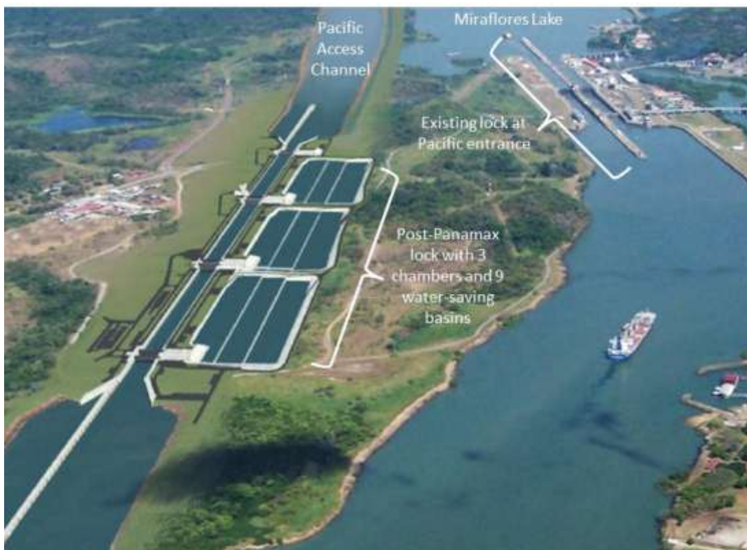
Figure 21: Design for Post-Panamax Locks, View from Pacific Entrance
